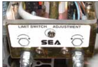
Mechanical limit switches screw adjustable
