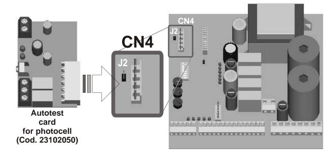
The CN4 connector can be used only to insert the autotest card for photocell (code 23102050); for the setting up make reference to the assembling instructions of the product itself. The autotest card mentioned above checks the good working of max two couples of photocells before every opening and closing. In case one of the two couples of photocells does not work correctly this card stops the equipment not allowing the opening or the closing.
