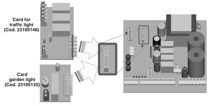
The CN5 connector can be used to insert the flashing lamp card (code 23105146) to which it is suggested to combine always the SEA two-lights flashing lamp (code 23105150) or to insert the garden lights card (code 23105135) which manages 100W max with a changing time (trimmer) from 60 to 120 seconds.
