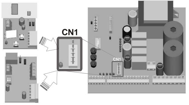
Notice: This connector is used only for the rapid connection of SEA designed products. Connector used for the rapid connection of inserting receivers or of the Decoder Module with keyboard.
