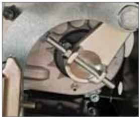
Adjustable mechanical stop in opening and closing
