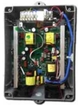
Battery back-up with fan cooling systems in option for AC motors
