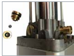
Hydraulic locks easy to change for maintenance
