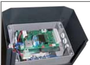
Electronic control unit positioned on the top of the carter
