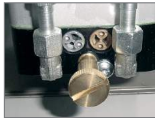
By pass valves for the force adjustment
